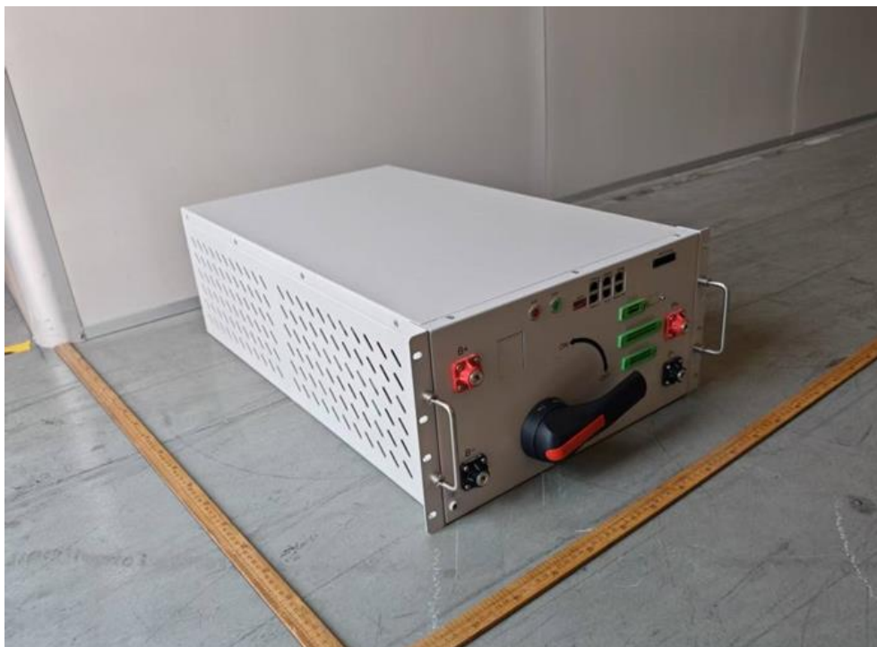
Figure 8 External view of high voltage control box
