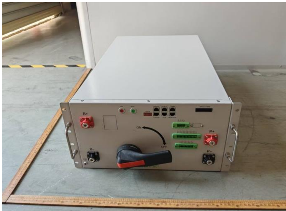
Figure 7 External view of high voltage control box
