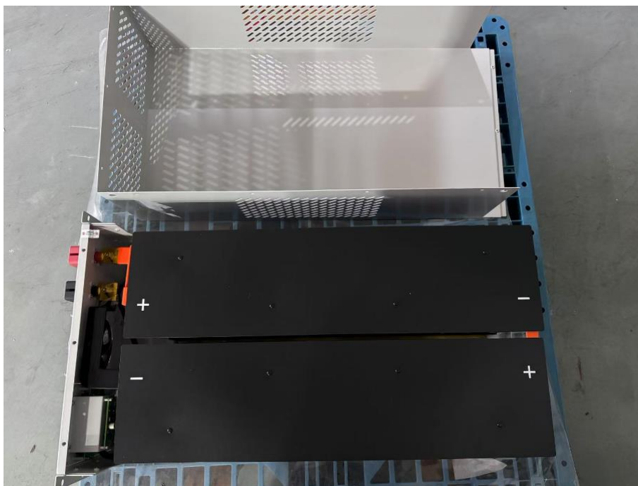
Figure 19 Internal view for battery module
