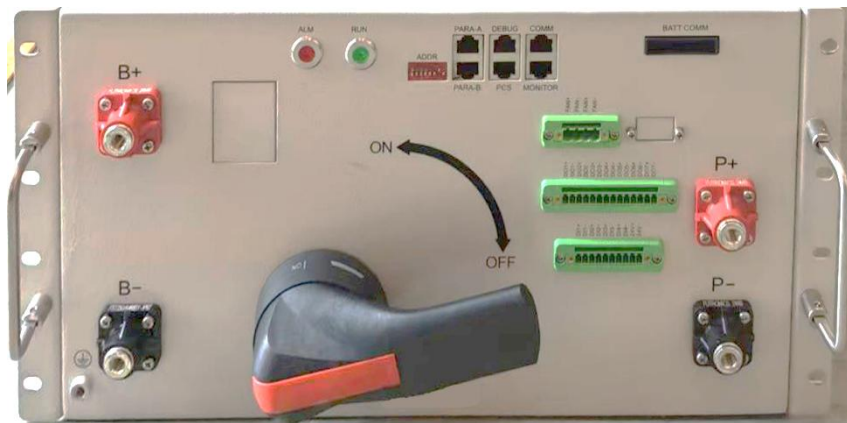
Polarity terminals of the battery system
