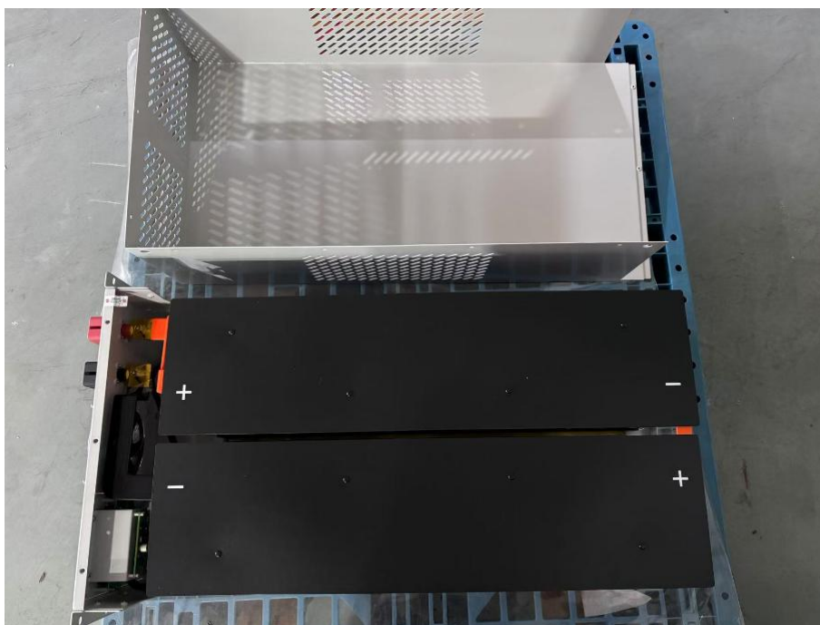
Figure 19 Internal view for battery module
